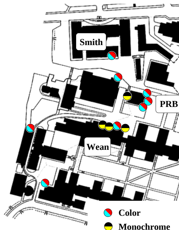
Figure 8: Placement of color and monochrome cameras in current VSAM testbed system. Not shown are two additional cameras, a FLIR and the SUO portable system, which are moved to different places as needed.
