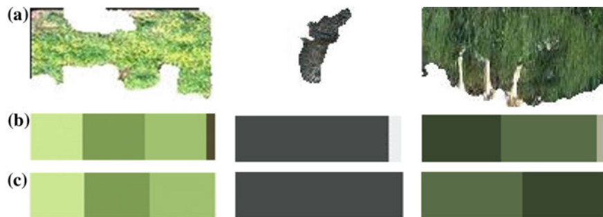
Fig. 4.23 Removal of noisy colors from segmented regions. a Three sample regions; b dominant colors of corresponding regions above; c DCDs after discarding insignificant colors from (b)
