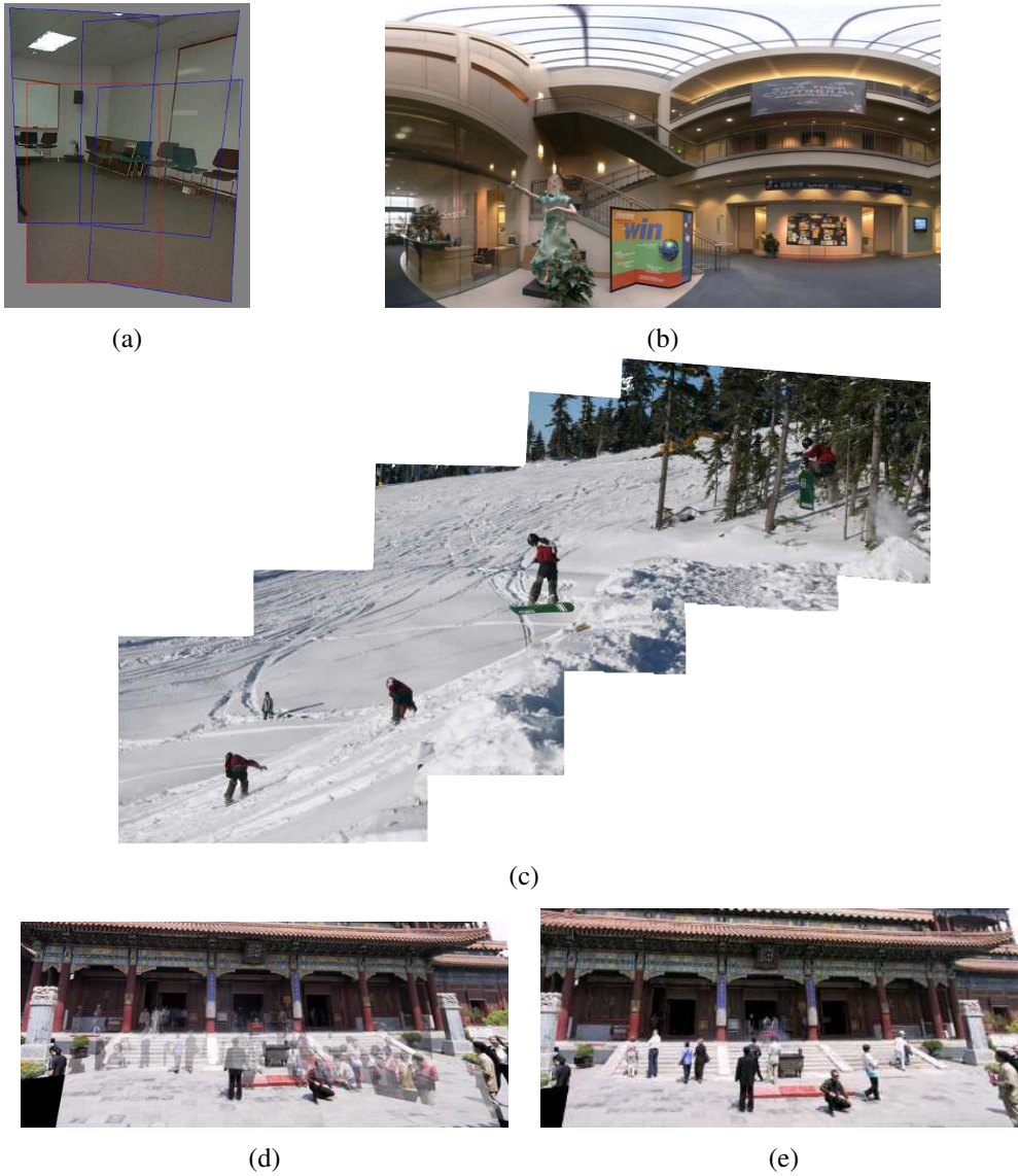
Figure 8.1 Image stitching: (a) geometric alignment of 2D images for stitching (Szeliski and Shum 1997) © 1997 ACM; (b) a spherical panorama constructed from 54 photographs (Szeliski and Shum 1997) © 1997 ACM; (c) a multi-image panorama automatically assembled from an unordered photo collection; a multi-image stitch (d) without and (e) with moving object removal (Uyttendaele, Eden, and Szeliski 2001) © 2001 IEEE.
