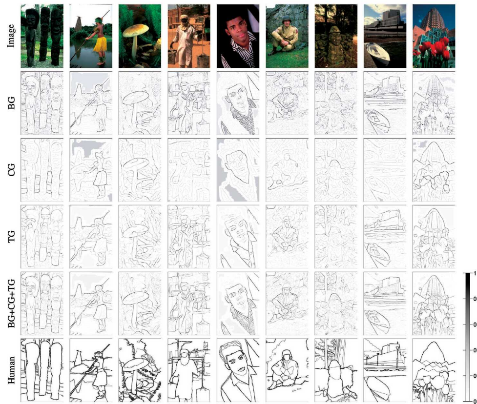
Figure 7.34 Combined brightness, color, texture boundary detector (Martin, Fowlkes, and Malik 2004) © 2004 IEEE. Successive rows show the outputs of the brightness gradient (BG), color gradient (CG), texture gradient (TG), and combined (BG+CG+TG) detectors. The final row shows human-labeled boundaries derived from a database of hand-segmented images (Martin, Fowlkes et al. 2001).
