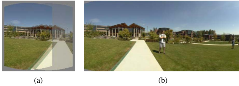
Figure 8.9 A cylindrical panorama (Szeliski and Shum 1997) © 1997 ACM: (a) two cylindrically warped images related by a horizontal translation; (b) part of a cylindrical panorama composited from a sequence of images.
