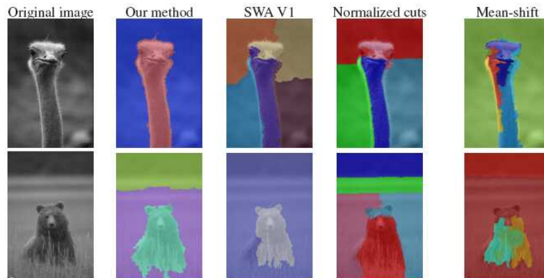
Figure 7.56 Comparative segmentation results (Alpert, Galun et al. 2007) © 2007 IEEE. “Our method” refers to the probabilistic bottom-up merging algorithm developed by Alpert et al.
